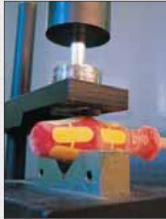
The Wera plastic material guarantees that the screwdriver passes the toughest low-temperature impact tests.
